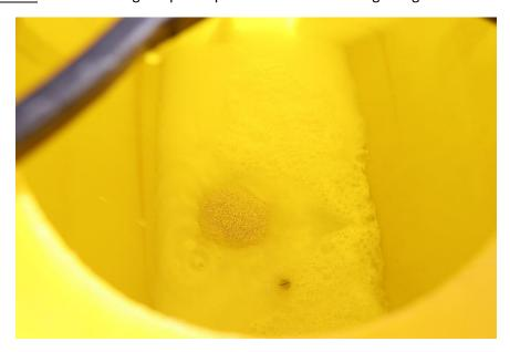
**STEP 6:** After Dr. Beck completed filling the tank with 100 gallons of water, we fashioned a ladle so we could reach into the bottom of the tank to determine how much if any product remained at the bottom of the tank.
